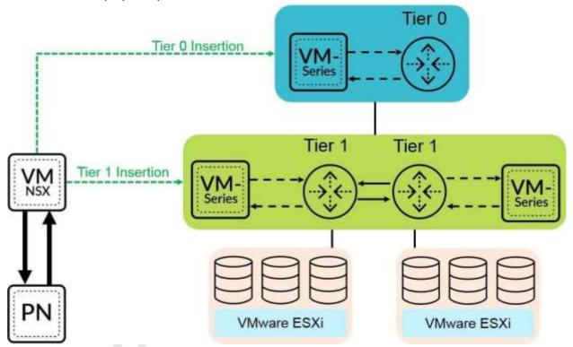
Tier-0 Insertion—Tier-0 insertion deploys a VM-Series firewall to a tier-0 logical router, which processes traffic between logical and physical networks. When you deploy the VM-Series firewall with tier-0 insertion, NSX-T Manager uses the deployment information you configured on Panorama to attach a firewall to a tier-0 logical router in virtual wire mode.
